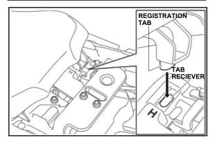
NOTE: It is normal for the front seat to press slightly on the OEM under seat body work in the low position. As an option, this body work may be trimmed slightly (2-3 mm) to alleviate this conflict.
