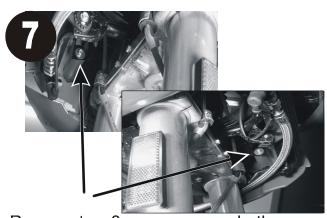
Remove two 8mm screws on both undersides of front panels.
