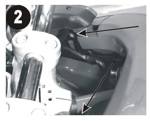
On right and left side panels, remove the two 8mm screws.
