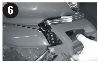
Pull the nose piece straight out of its two snap-in pins.
