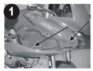
On right side panel, remove the two 4mm screws.
