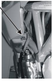
On the left side panel, pull out the slide clip. Next pull the side panel off its two pressure studs.
