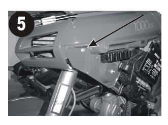
On the left side only, remove the 4mm screw.
