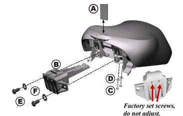
Place support bracket (B) into opening at the rear of the seat.
